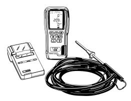
The C100A enables HVAC professionals to accurately test and service all residential combustion appliances. The extra large backlit LCD dislays three parameters at one time. The C100A can store, retrieve, view and print up to 99 test results. The optional printer allows you to print a copy of all your readings right on the spot to document your test results.
